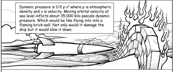
At 100 km altitude the air's so thin the ship suffers little dynamic pressure. Ships usually attain this altitude before doing the major burn to achieve orbital velocity.
