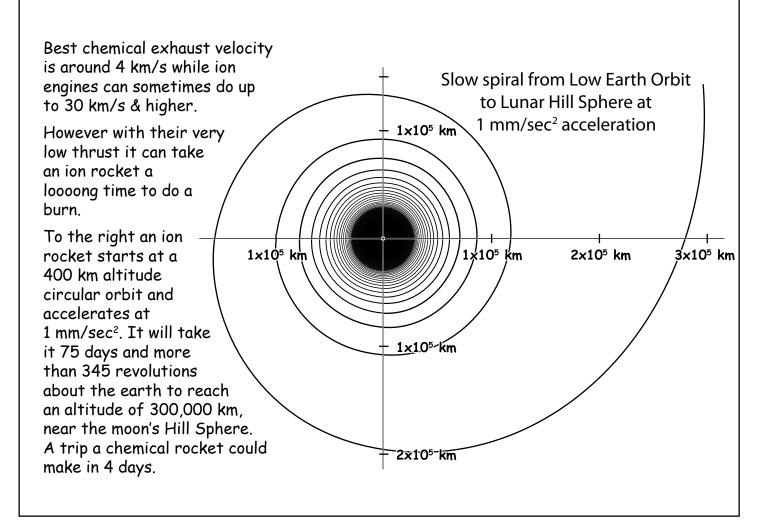
Ion engines can have a much higher exhaust velocity but with the lower acceleration it takes much longer to achieve a change in
