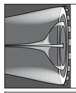
In a darkened room the plume of ionized xenon coming from an XR-100 Hall Thruster is a beautiful thing to behold. The ionized xenon atoms go in different directions at different speeds but the effective exhaust velocity ranges from 16 to 32 km/s.
